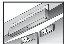
The mounting plate should be screwed to the L-bracket prior to installing the L-bracket. After the L-bracket is installed the magnet can then be screwed to the L-bracket.
