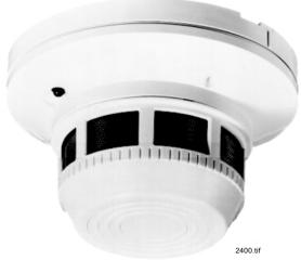
The built-in piezoelectric horn produces an interrupted 85 dBA tone. The horn operates when the unit senses smoke, or when the thermal reaches its alarm point (integral thermal models only).
