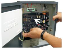
Connect the **mains cable** directly to terminals on the Retrofit MRC.
