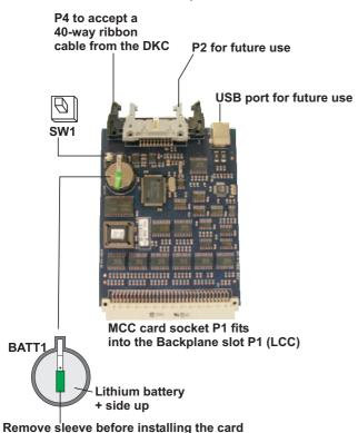
Once the battery sleeve is removed from the MCC, the card MUST NOT be placed on a metal surface as this may result in damage to the components on the card.
