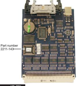
This MCC MUST NOT be installed in BS version of Vigilon or 34000 Fire panel.
