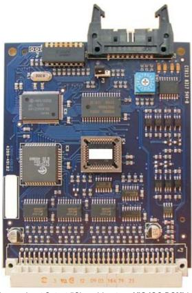
The new Input Output (IO) card (part no. VIG-IOC-DOM) is designed for installation in EN54 Vigilon analogue addressable fire panels and Network node:
