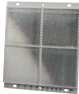
The 6500RE and 6500RSE are conventional reflector type linear optical beam smoke detectors designed to operate as a component of a non-addressable fire alarm system. It operates primarily on the principle of light obscuration utilising infra-red light. Optical beam smoke detectors are particularly appropriate for protecting buildings with large open spaces such as warehouses, atriums etc.
