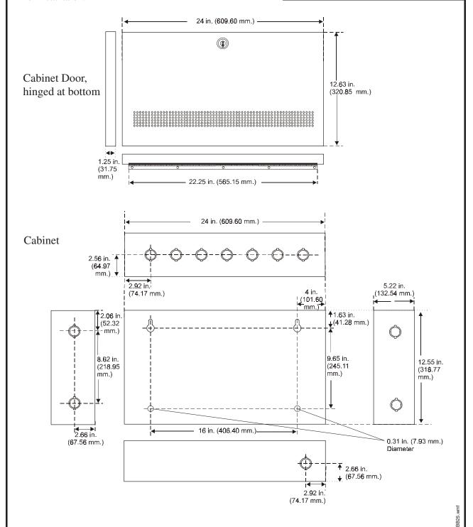
The BB-25 Cabinet comes with a false bottom plate. Place this plate in the bottom of the cabinet for battery support.
